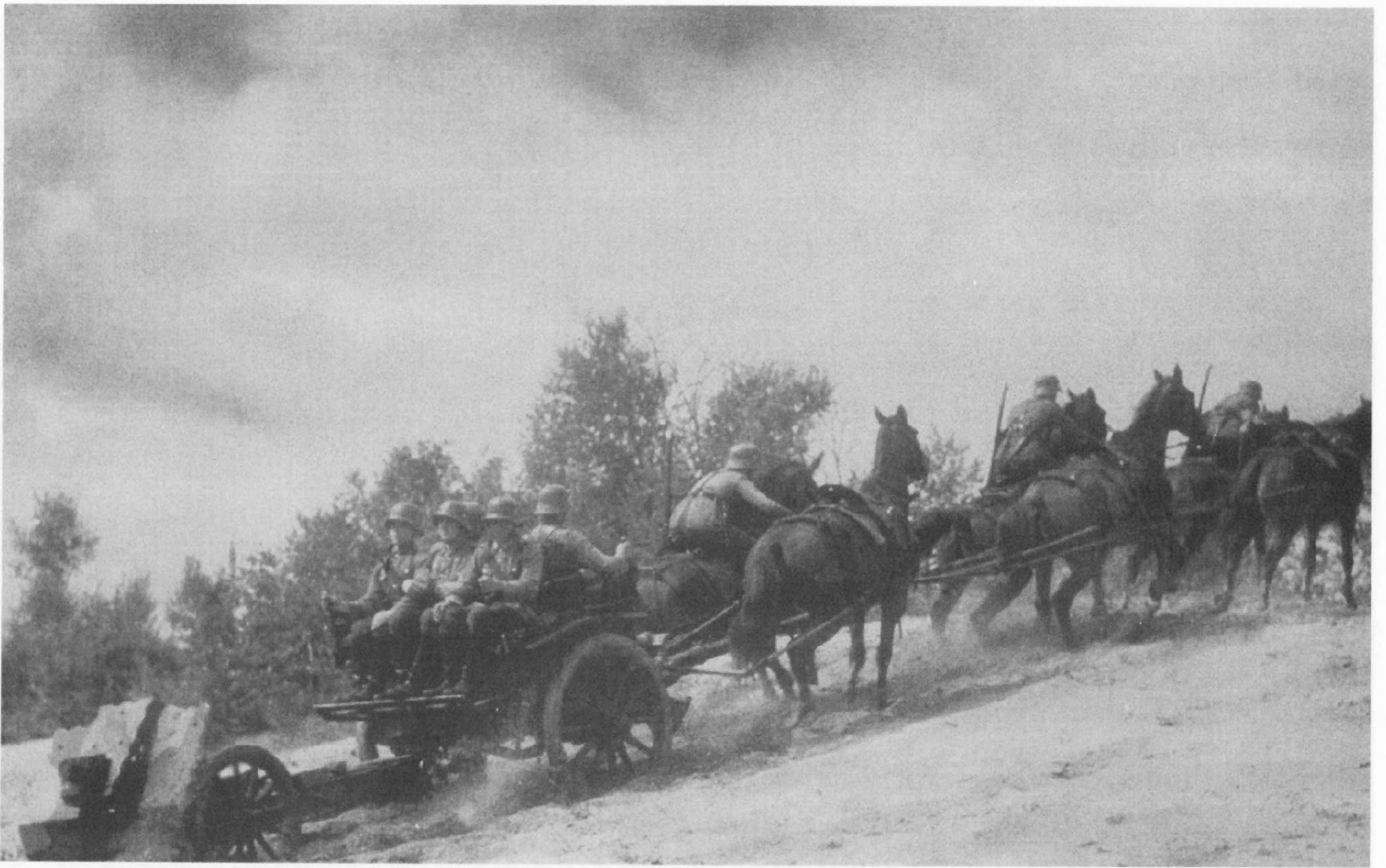
In the horse regiments the cavalry gun was pulled by a team of six horses. Accordingly it and its associated front limber were fitted with spoked wheels.
